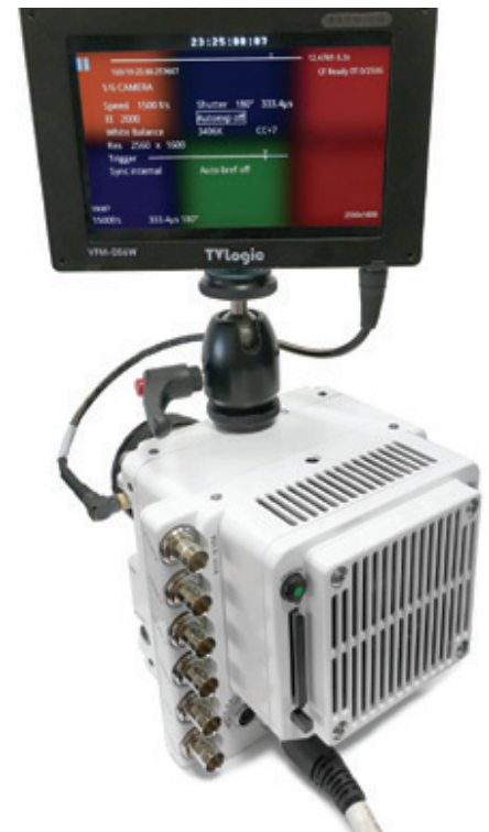
Phantom VEO-S with monitor and CFast 2.0 card, displaying the on-camera control menu
